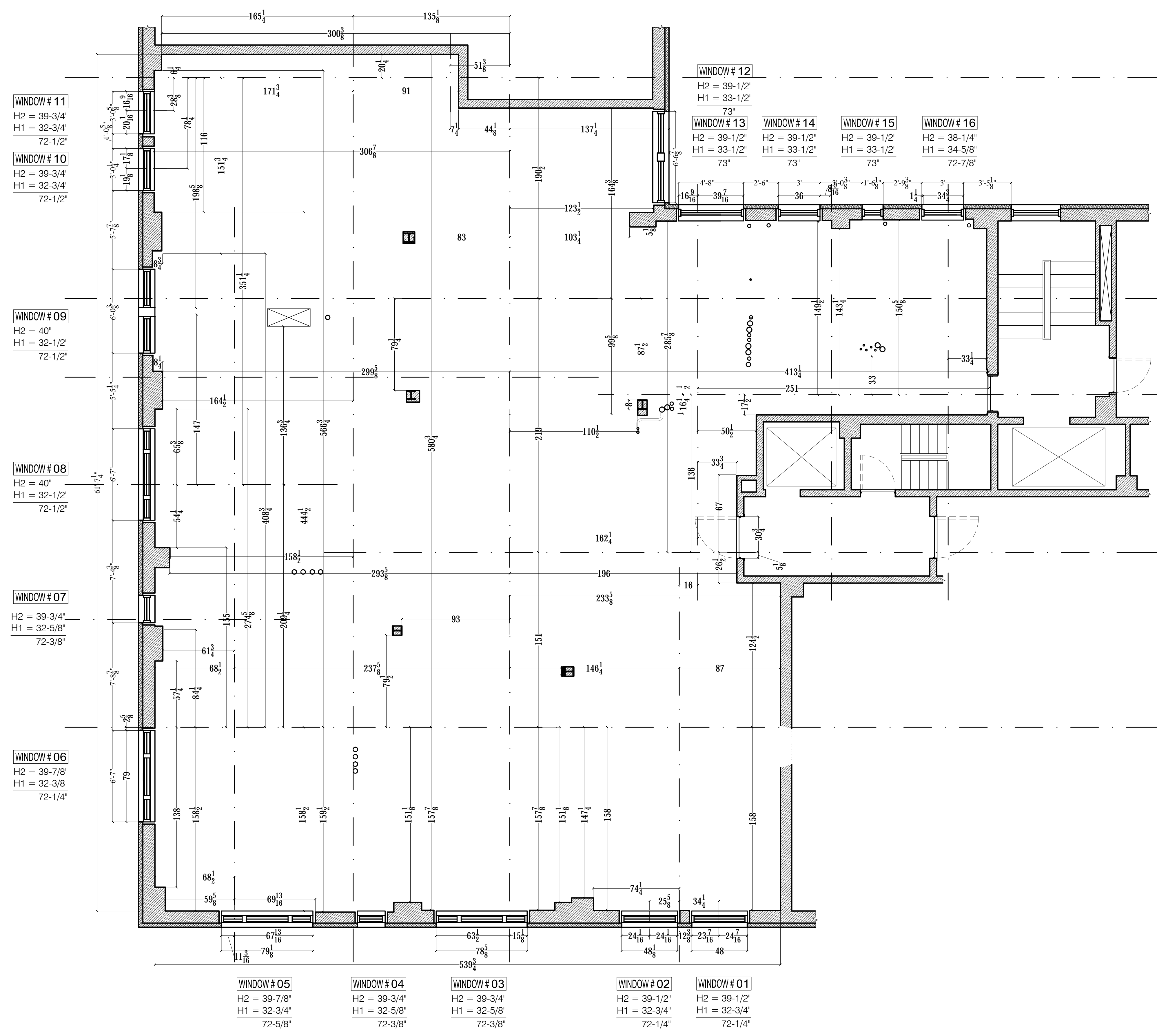
1 SURVEY PLAN - EXIST'G WALL & WINDOWS 1/4"=1'-0"
